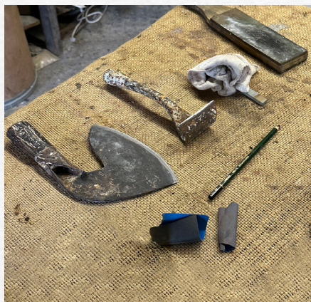
Tools used for harvesting natural lacquer sap.
